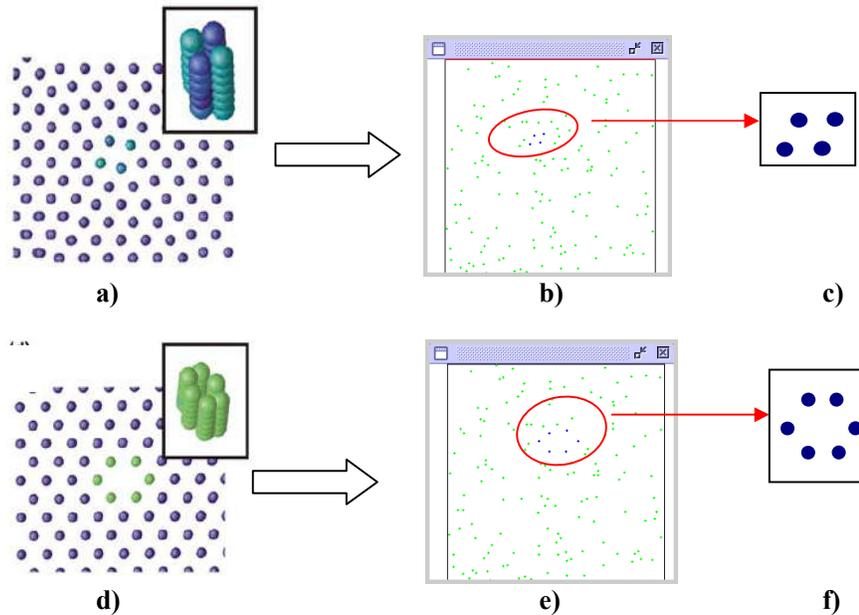
**Fig. 1.** Schematic model of two dislocation process: a) trail of partial point defects, d) vacancy tube [Buehler et al., 2005], b) trail of partial point defects, e) vacancy tube, our generated models, c) and f) 2D section through the dimensional elastic field for both cases.
