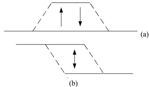
Fig. 3. The elementary states for the dislocation movement: a) migration and pair of nodes formation, b) pair of nodes annihilation
