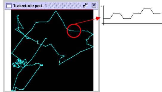
Fig. 2. Trajectories for the partial point defects for one atom of the trail and the kink model of the dislocation lattice
